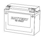
Endurance II. A 0.5A fuse (not provided) should be used between the power cable and positive battery terminal when connecting directly to a battery.
